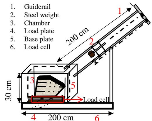
Fig1. Drop weight falling impact test
