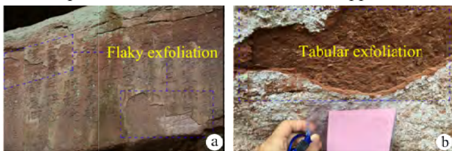
Fig. 1 a Flaky exfoliation; b tabular exfoliation (There is the sampling point of weathering sandstone samples. The thickness of tabular exfoliation is approximately 10 mm.)
